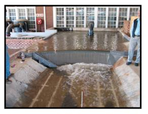
Figure 2.1: Neckartal Dam Spillway Model
