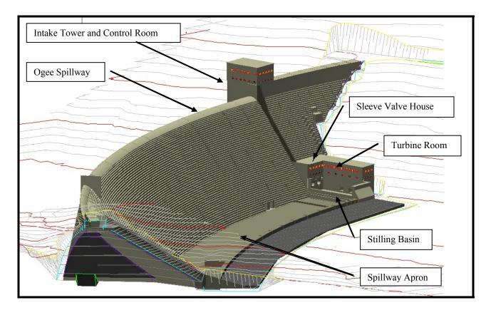
Figure 1.1: Neckartal Dam (Isometric view)
