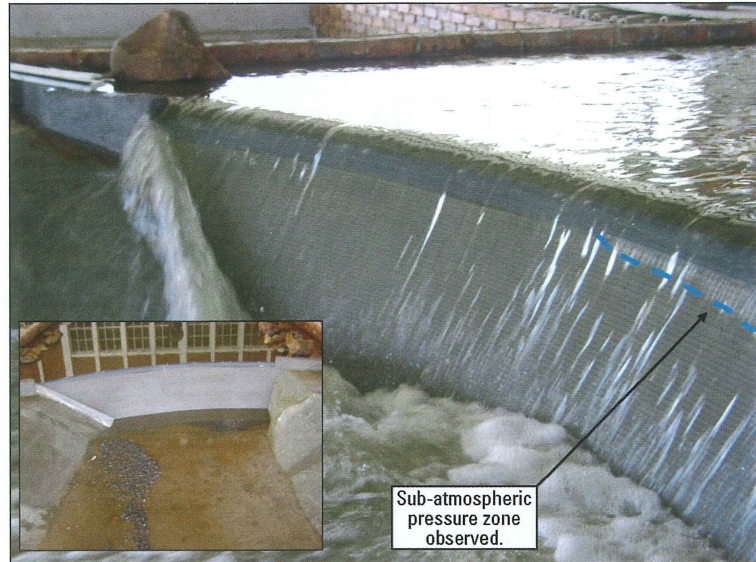
Fig. 5. Flow accentuated towards the downstream wall of the chute. Unacceptable high flow depths were experienced in the chute. Breakaway was also observed towards the left bank of the spillway (Inset: Significant erosion and large recirculation flow present during the RDD).
