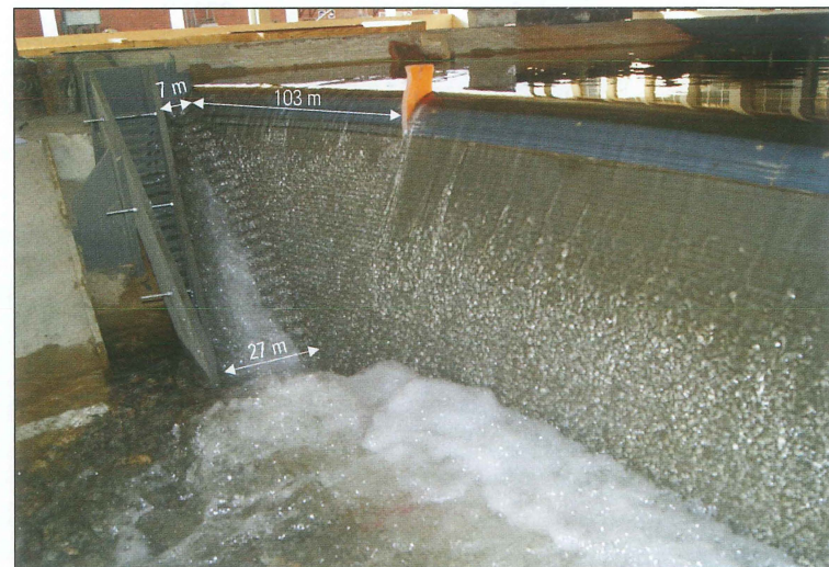
Fig. 6. Option 4: Flow depth on the spillway chute during the RDD. The last 103 m of the Ogee crest was raised by 2.4 m and the dimensions of the chute were 7 m on the top and 27 m at the bottom.
