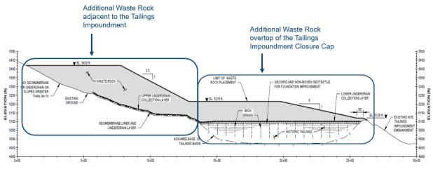
Figure 10 Conceptual Closure Enhancement – Waste Rock Storage Area
