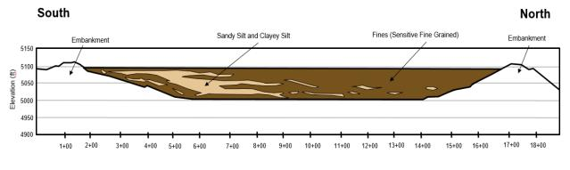
Figure 5 Typical South-North Stratigraphic Section through the Nye Tailings Impoundment
