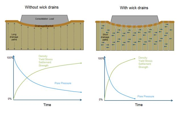
Figure 9 Schematic ground improvement technology consisting of a compressive load constructed over tailings amended with wick drains.
