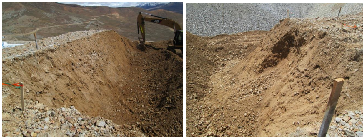
Figure 12: Excavations performed after completion of the leaching test, a homogeneous moisture distribution along the profile of excavations were observed
