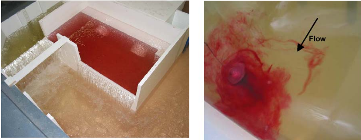
Figure 13: Model test - Flow through the Discharge Chamber and Tailrace and over weirs (left). Vortex appearing as submergence above the outlet decreases (right).
