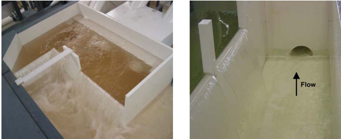
Figure 14: Model test - Flow through the Discharge Chamber and Tailrace and over weirs (left). Flow (spill) over overflow weir into overflow channel to spillway.
