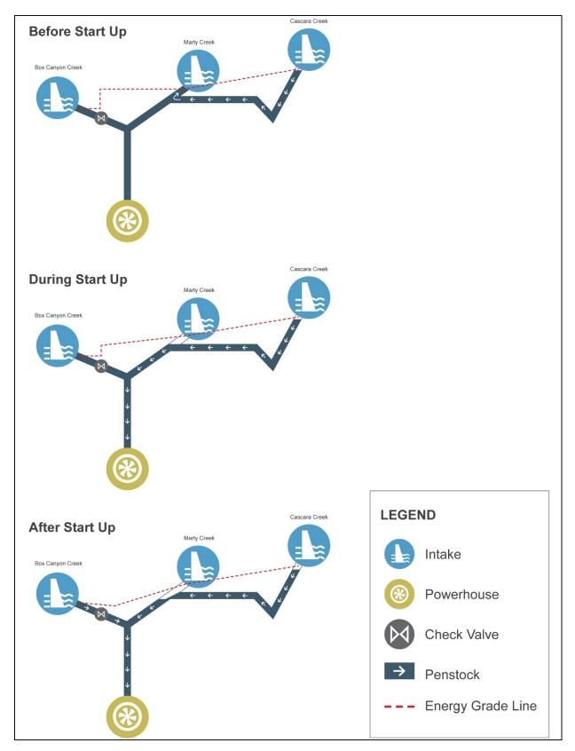
Figure 5: Head and penstock water level before, during and after start up.
