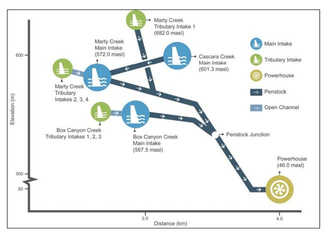
Figure 4: Intake elevation and penstock length schematic.
