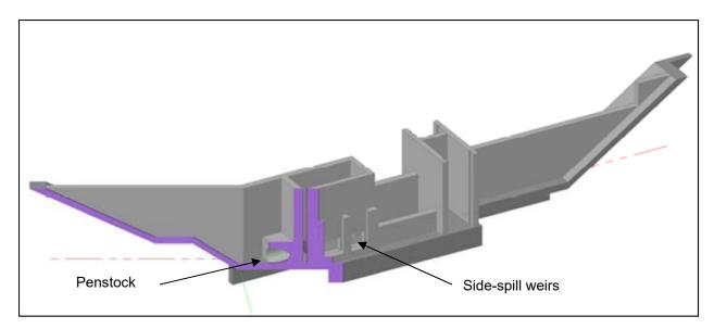
Figure 3: Isometric view of Marty Creek intake concrete works showing the sidespill weirs, which are used to control the maximum diversion rate.
