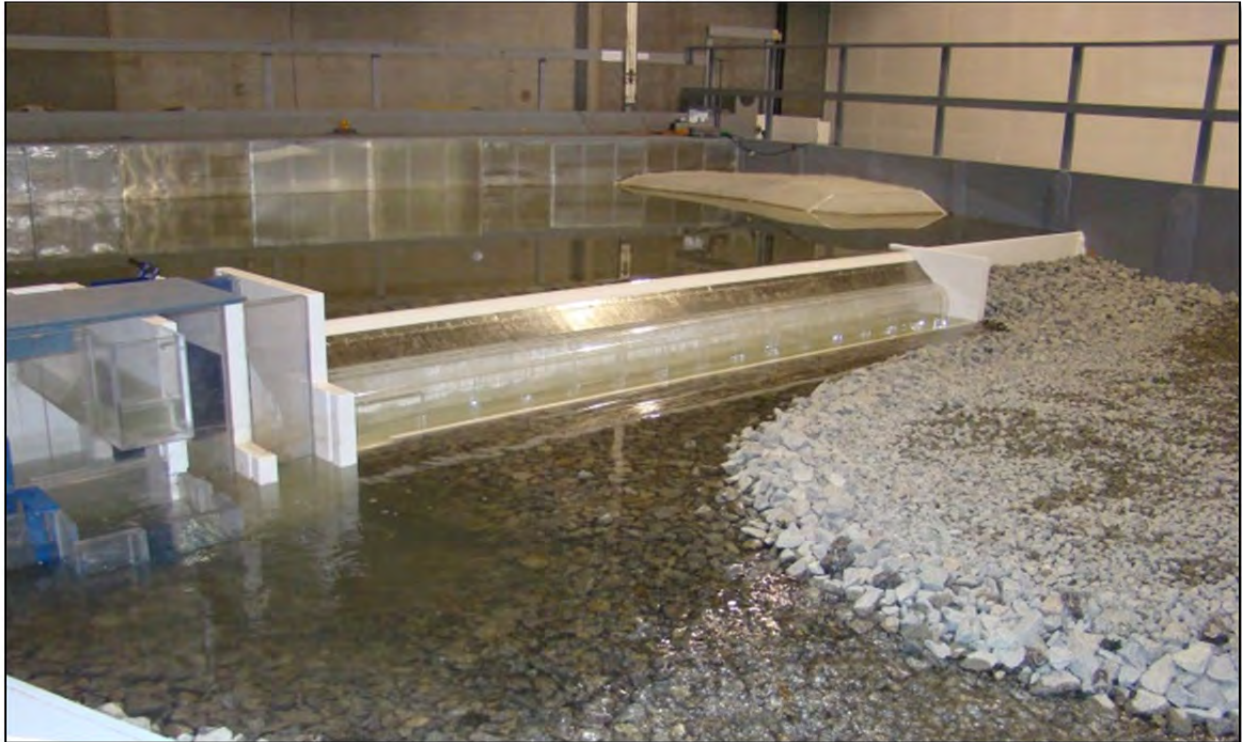
Photo 2: Kokish River HEP Headworks - Hydraulic Model
