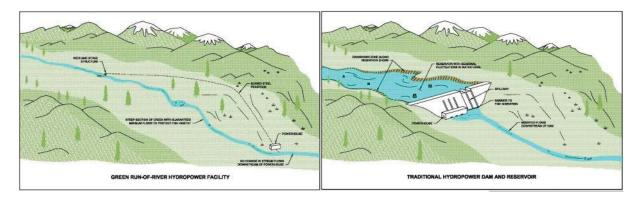
Figure 1. Schematic Layout of Large Dam and Run- of-River Hydroelectric Facilities
