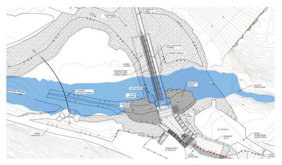
Figure 7. Kokish River Intake General Arrangement
