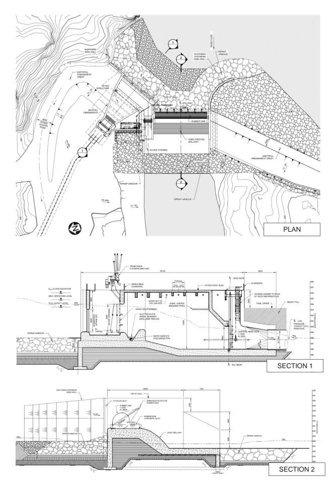
Figure 3. Reservoir De-sander Type Intake – Plan and Sections
