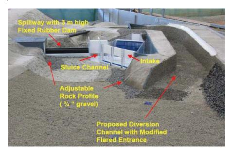
Figure 4. Physical Model Constructed and Tested for the 33 MW Upper Stave River HEF
