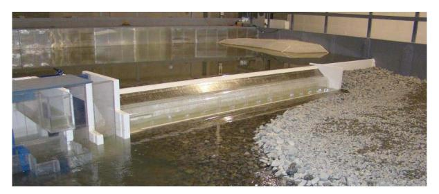
Figure 8. Kokish River Intake Physical Model
