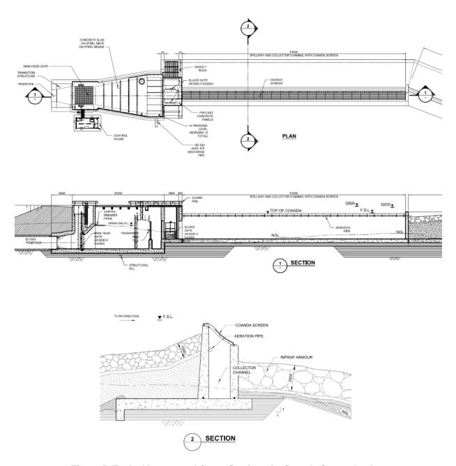
Figure 5. Typical Layout and Cross Section of a Conada Screen Intake
