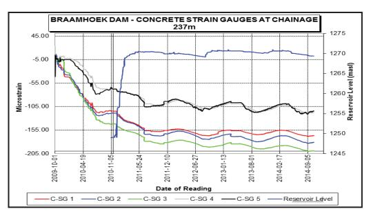
Figure 8. Bramhoek Dam Strain Gauge readings
