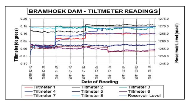
Figure 5. Bramhoek Dam Tilt Meter readings
