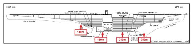
Figure 6. Bramhoek Dam Position of Piezometer rows
