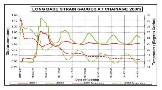
Figure 3. Braamhoek Dam LBSG at chainage 260m
