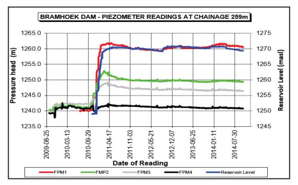
Figure 7. Bramhoek Dam Piezometer readings on the left bank
