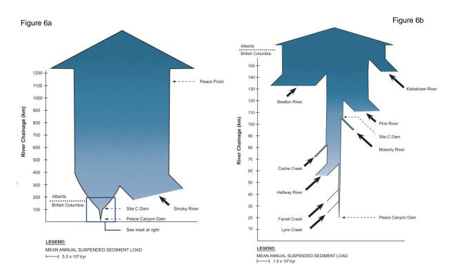
Figure 6 Peace River suspended sediment load.
