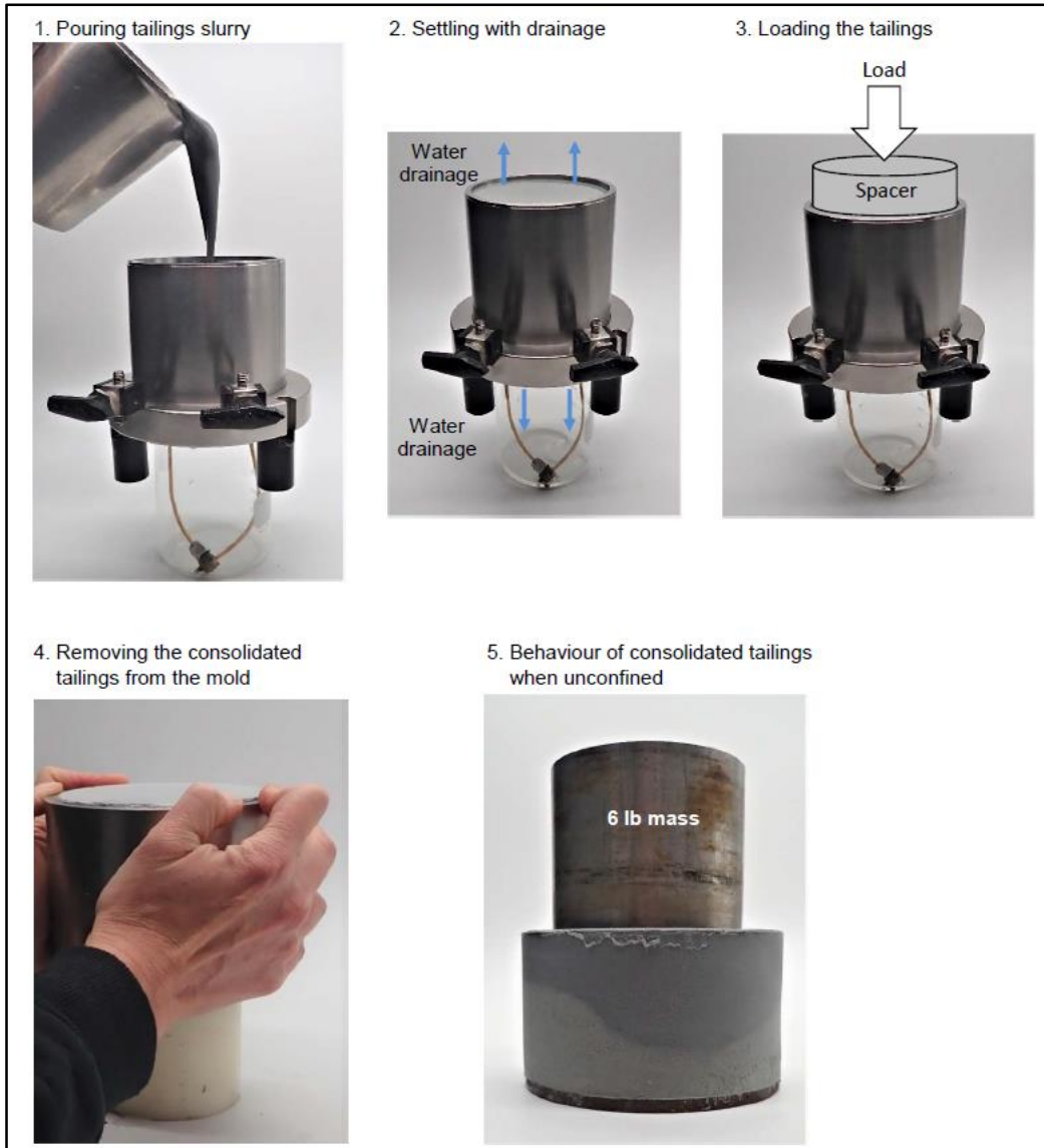
Figure 6 Tailings Slurry Consolidation Test – Photo Summary
