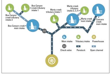
Fig. 2. Schematic highlighting the complexity of the Box Canyon project.
