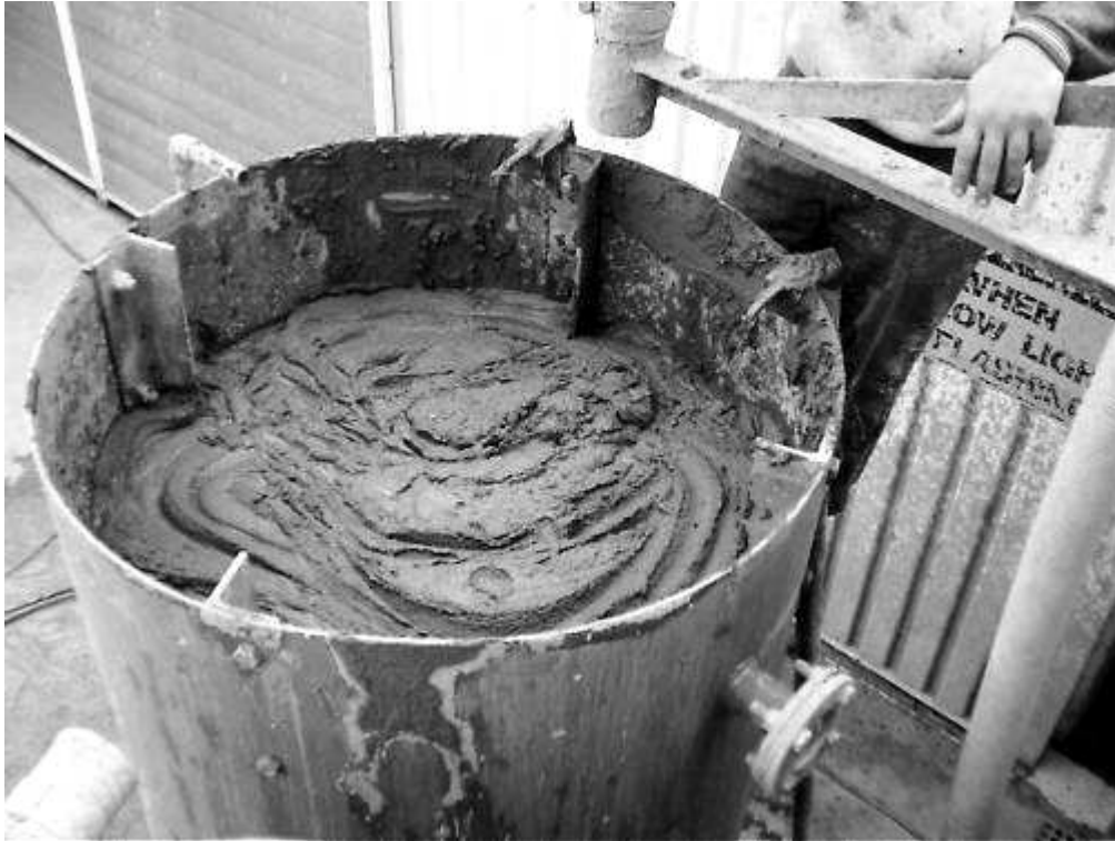
Figure 1 Non-Newtonian thickened tailings ( \tau_y = 70 Pa, K_b = 0.060 Pa.s)
