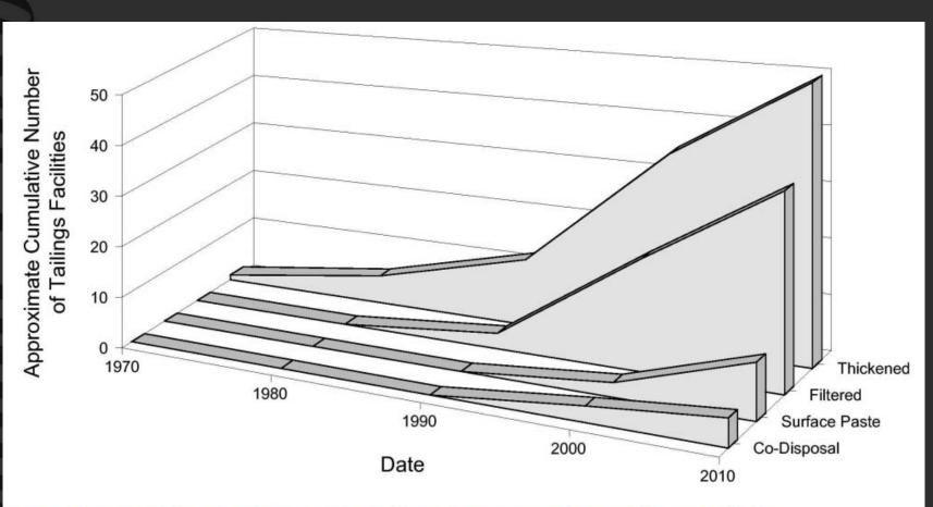
Figure 2: Trends in Use of Dewatered Tailings in Mining (after Davies et al, 2010)
