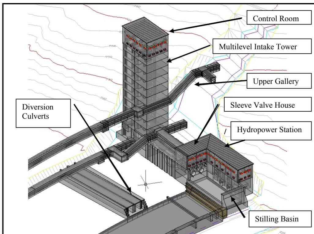
Figure 2: Neckartal Dam Outlet Works (isometric view)
