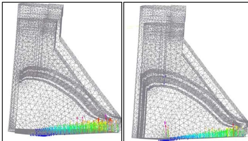
Figure 3: Maximum Operating Load Case with Two Compromised Anchor Scenarios Showing Less than 100% Compression
