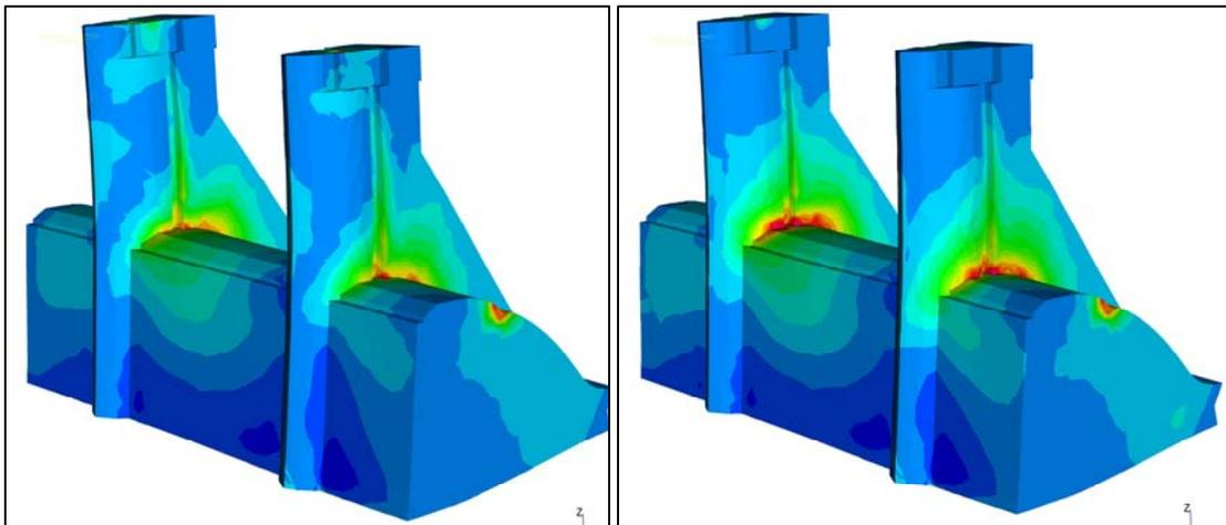
Figure 4: Longitudinal Ground Motion Mohr Coulomb Stress – With and Without Pier Anchors, Red Region Propagating When Compression in Piers from Post-Tensioned Anchors are not Considered
