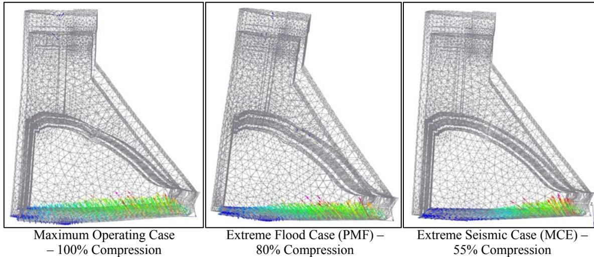
Figure 2: Overturn Base Compression Reaction Vectors – Max Operating vs. PMF vs. MCE
