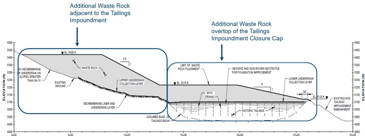
**Figure 10** Conceptual Closure Enhancement – Waste Rock Storage Area
