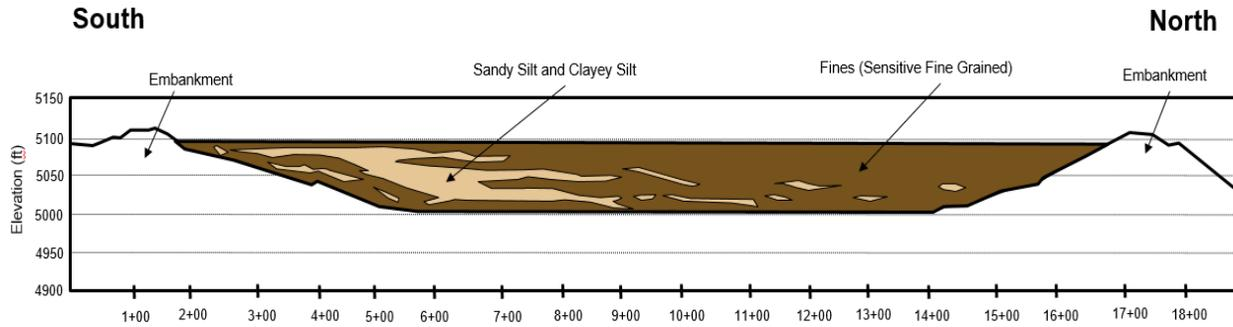
**Figure 5** Typical South-North Stratigraphic Section through the Nye Tailings Impoundment
