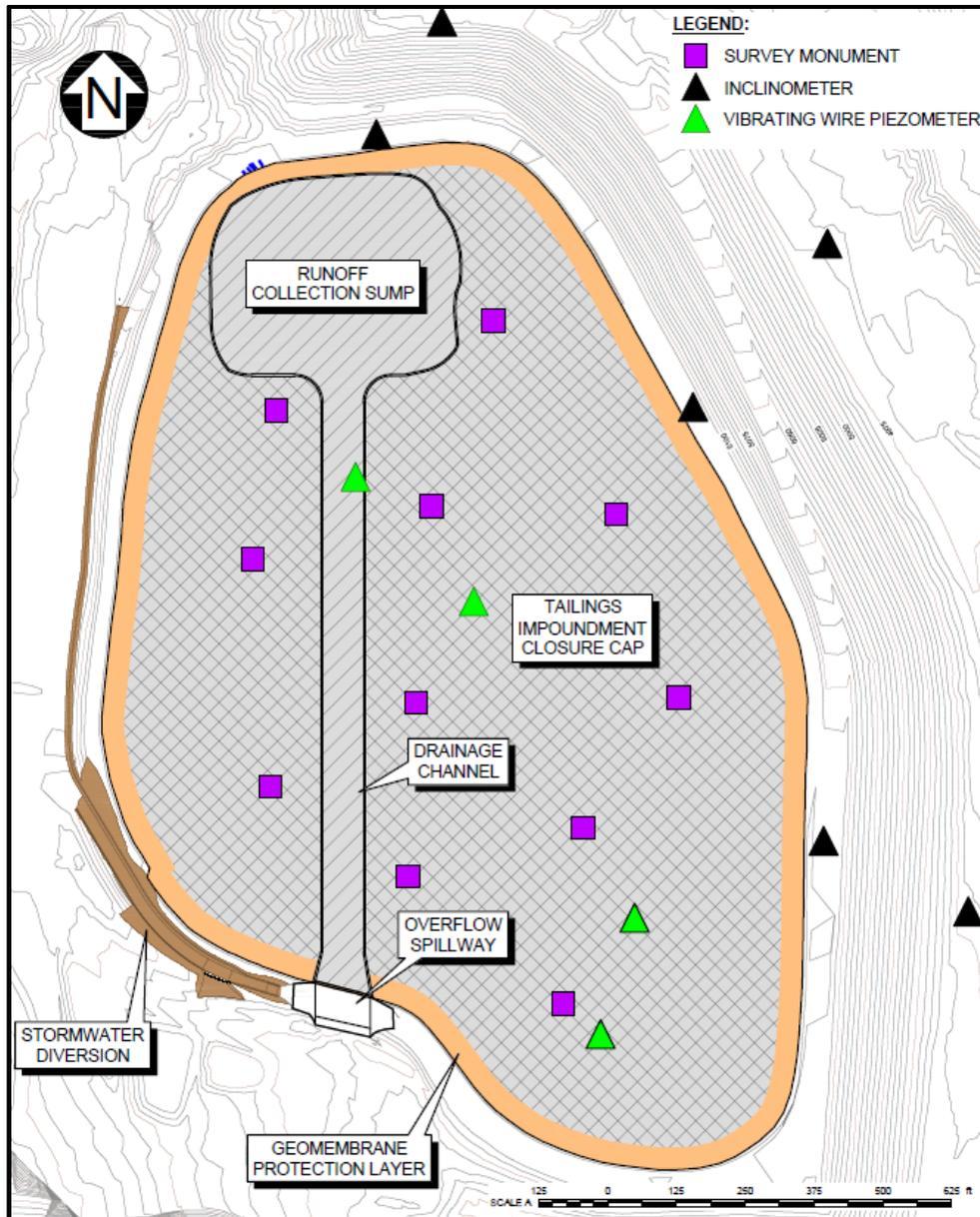
Figure 7 Closure Cap during Operations
