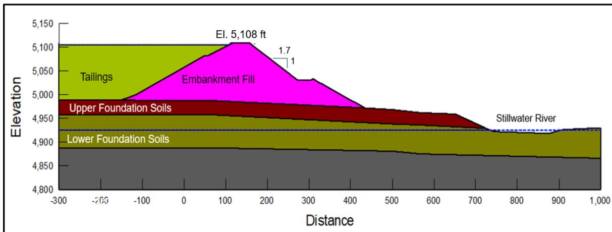
**Figure 3 Typical Embankment Cross Section**
