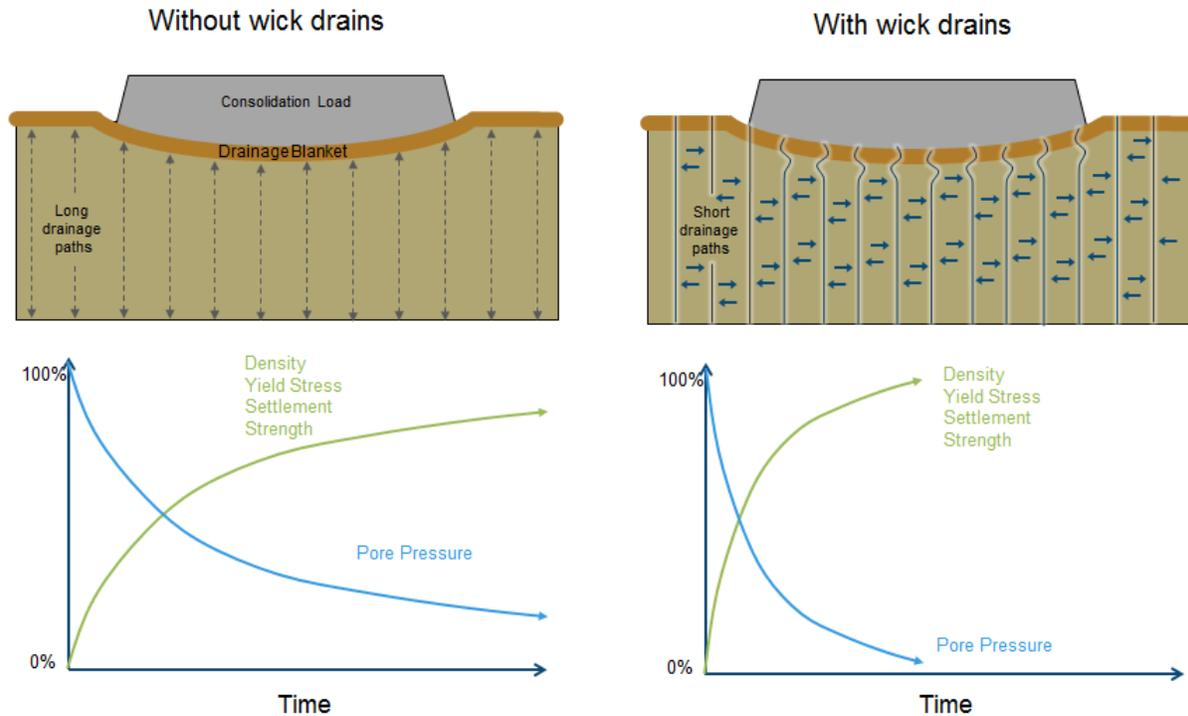
**Figure 9 Schematic ground improvement technology consisting of a compressive load constructed over tailings amended with wick drains.**
