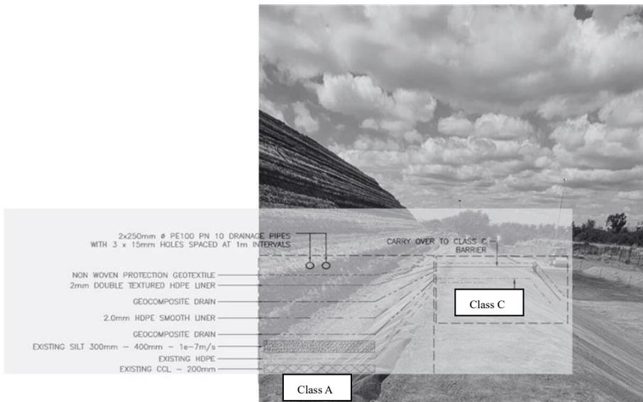
**Fig. 1.** New Class A and Class C barrier systems.
