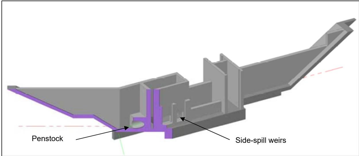
***Figure 3: Isometric view of Marty Creek intake concrete works showing the side-spill weirs, which are used to control the maximum diversion rate.***
