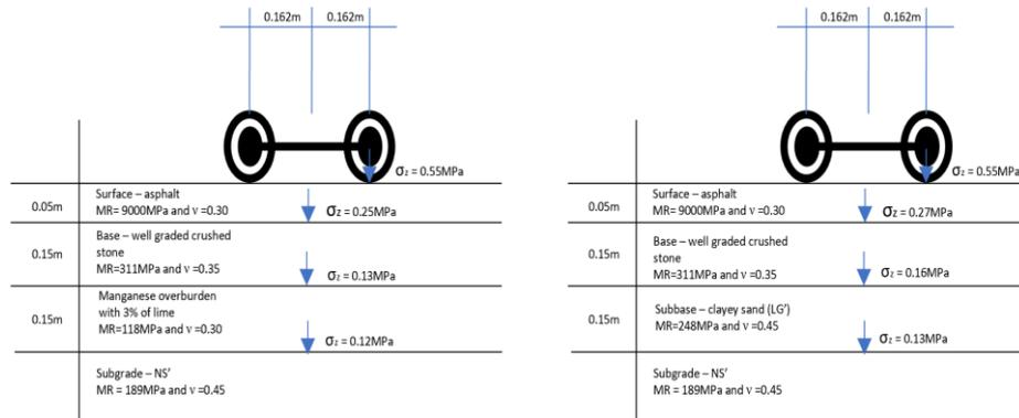
**Fig. 5.** Pavement cross-section with a lateritic clayey sand subbase (used in Brazil) and with a subbase composed of manganese overburden improved with 3% lime.
