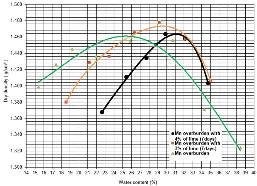
Fig. 2. Compaction curves – manganese overburden and manganese overburden-lime mixtures.
