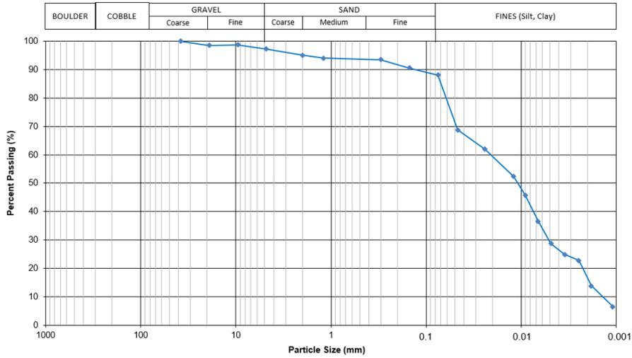
Fig. 1. Particle size distribution curve – manganese overburden.
