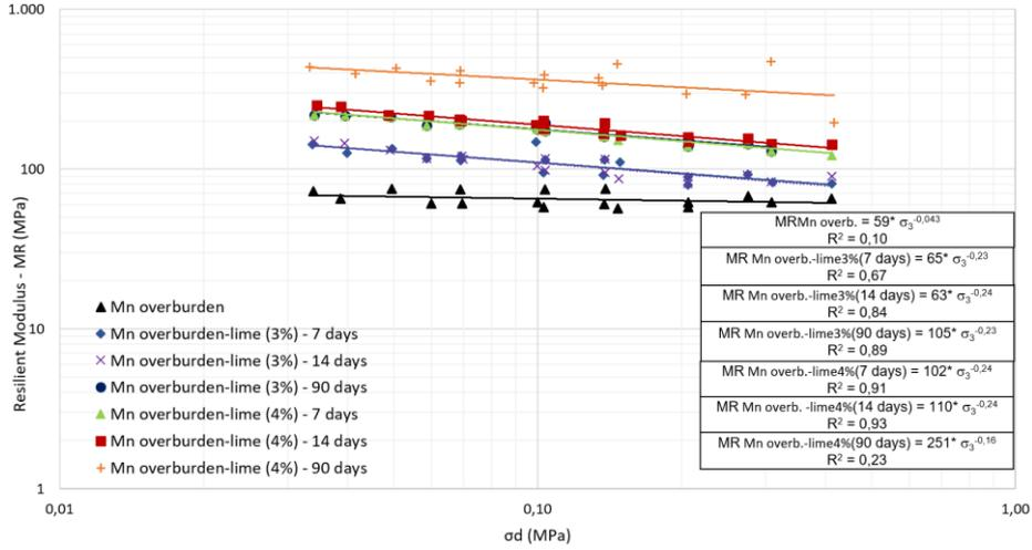
Fig. 3. Resilient modulus as a function of the deviator stress ( $\sigma_d$ ).
