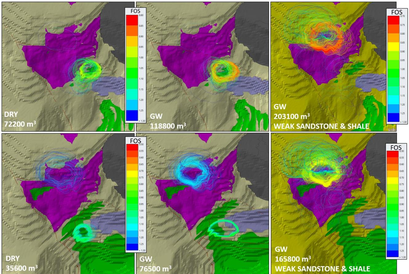
Figure 11. Areas of concern identified by limit equilibrium analysis, 2018 pit (top) and toe removal (bottom).
