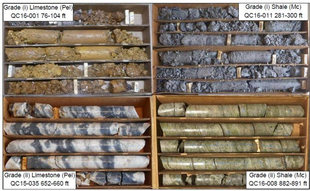
Figure 4. Comparison of rock mass quality between the alteration grades.
