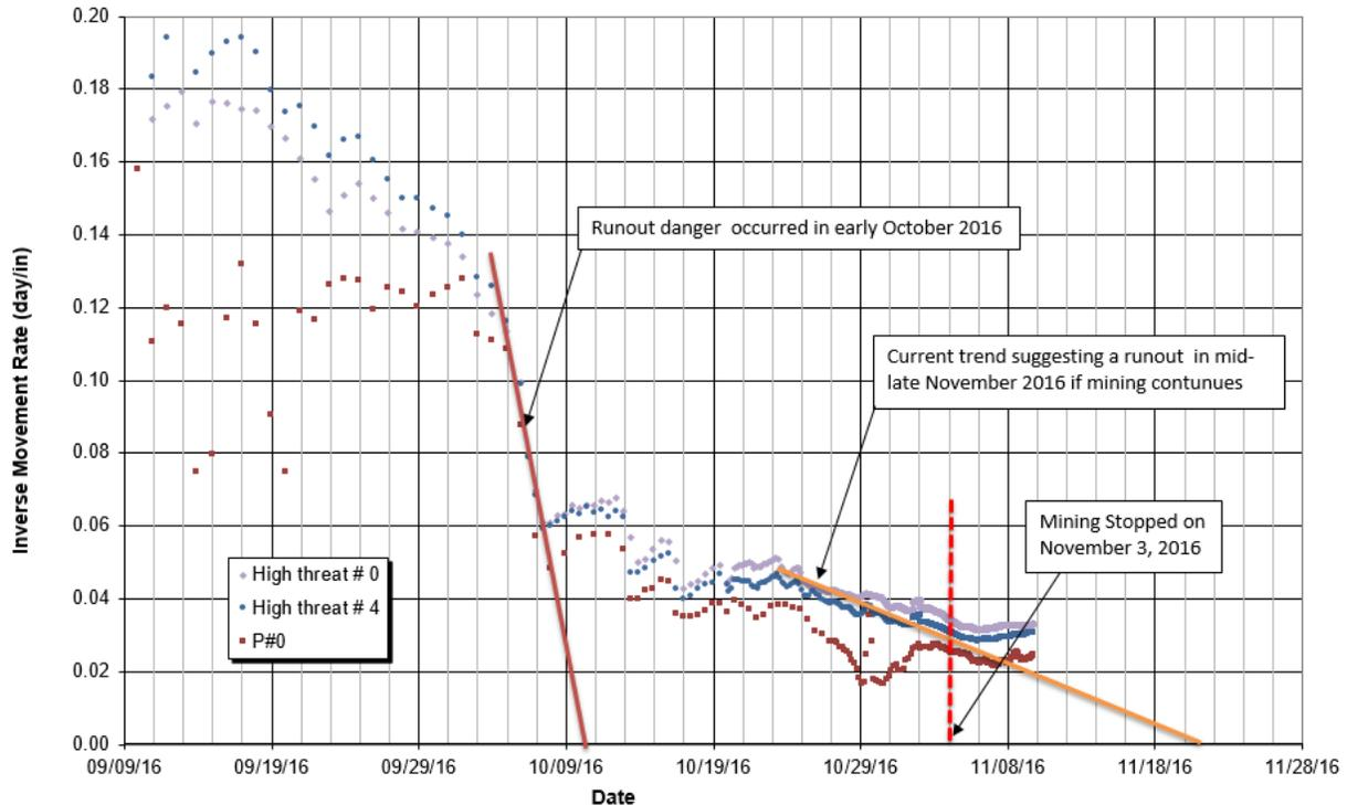
Figure 7. Inverse velocity trends of the north wall 2016 instability.
