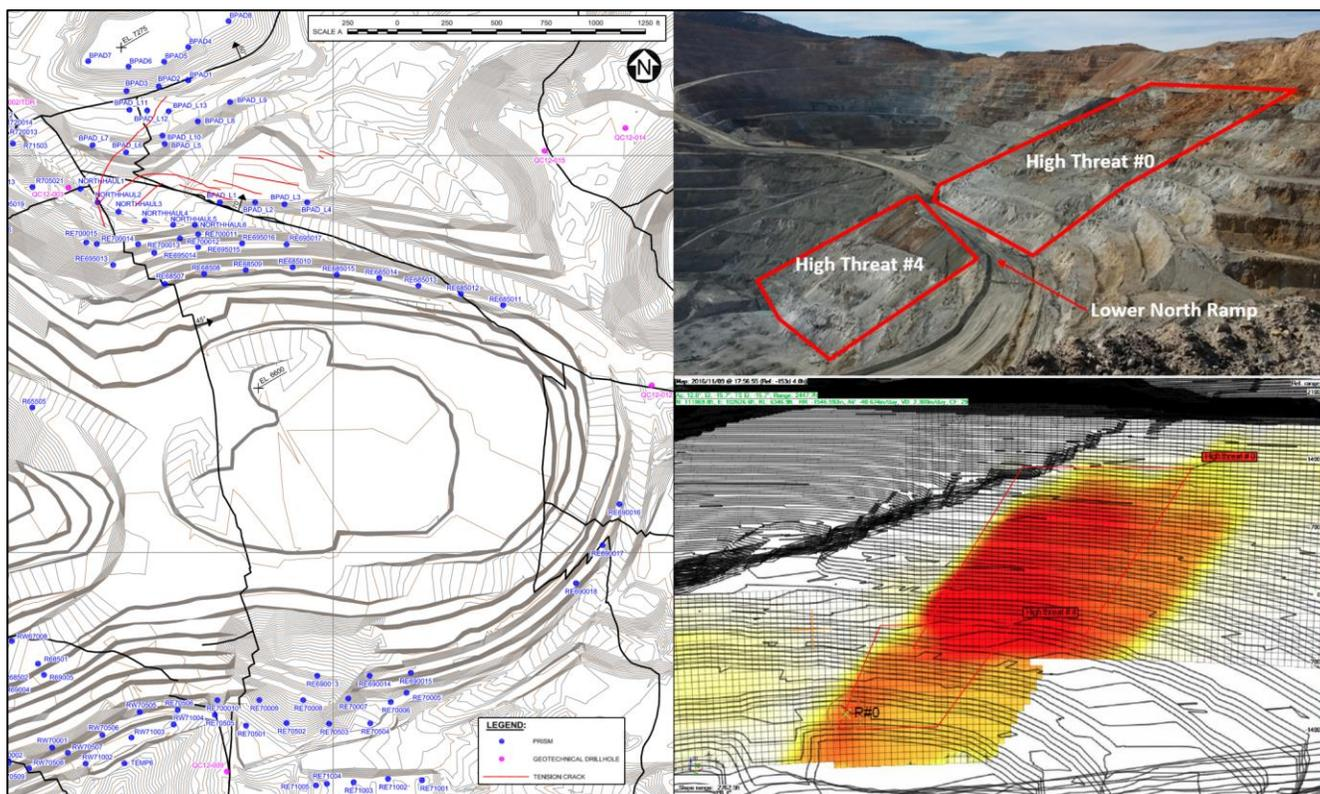
Figure 6. Displacement monitoring by survey prisms (left) and terrestrial radar (right).
