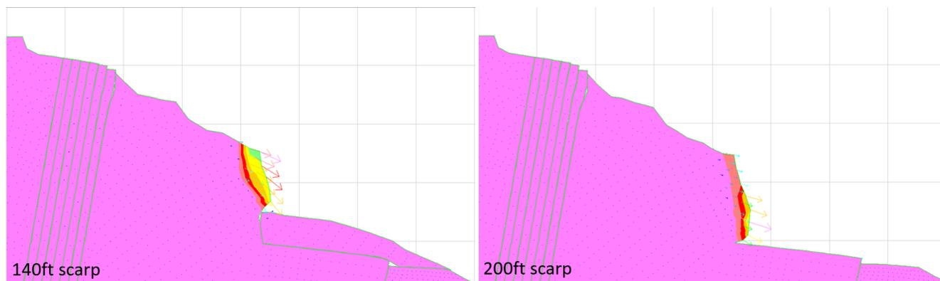
Figure 8. Predicted displacement magnitudes and velocity vectors of the back scarp.
