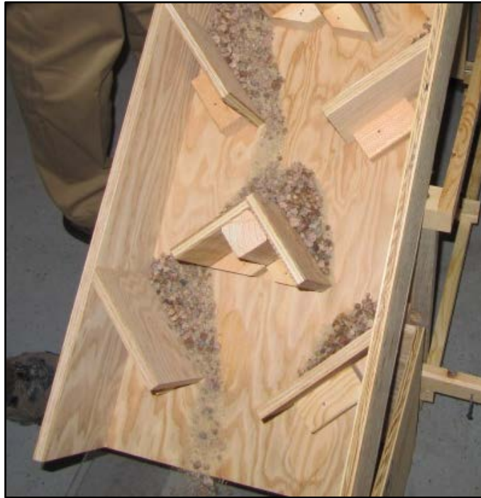
Figure 6: Static Mixing Device Showing Mixing of Materials
