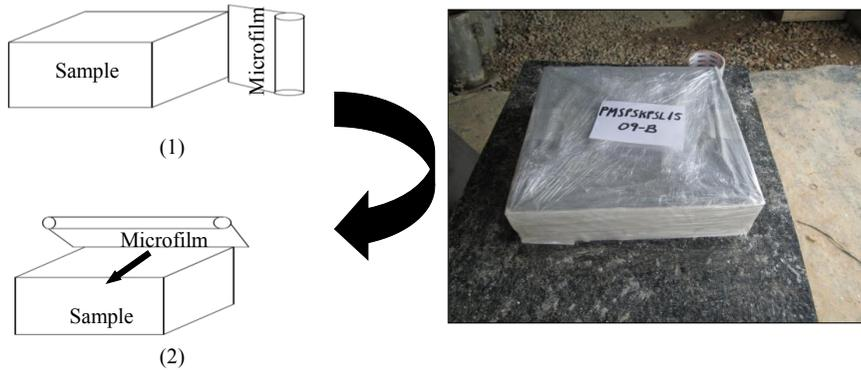
Figure 7. Placement of microfilm.
