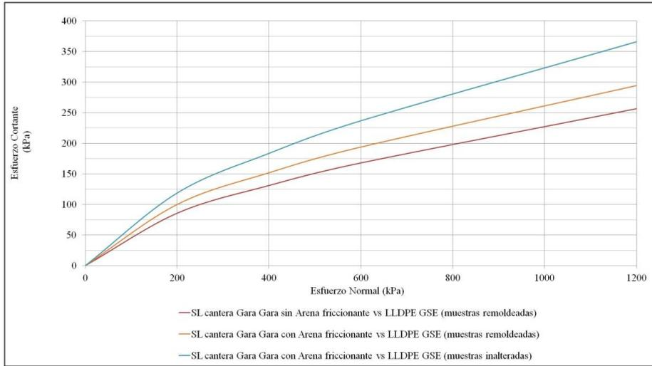
Figure 9. Envelopes of the interface tests of soil liner with friction sand vs. GSE geomembrane.
