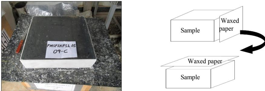
Figure 6. Parafining of the sample and placement of waxed paper.
