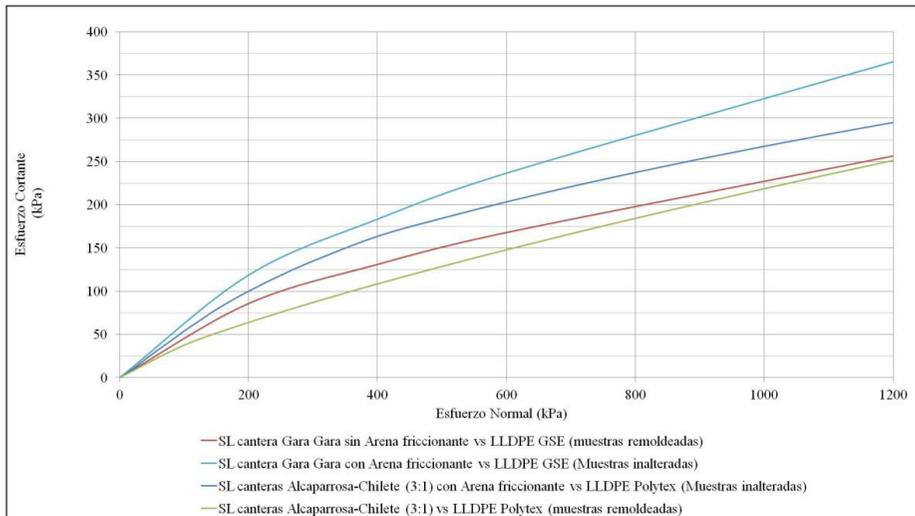
Figure 10. Envelopes of the interface tests of soil liner with friction sand vs. GSE and Polytex geomembranes.
