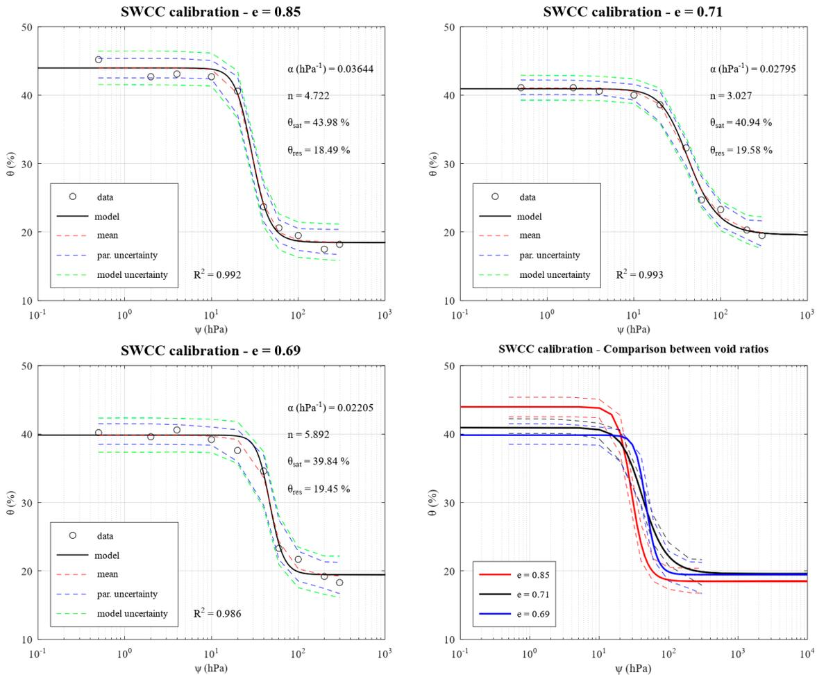
**Figure 1: Calibration of van Genuchten parameters**
