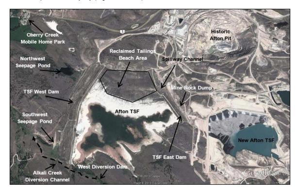
Figure 1. General arrangement of the Afton TSF
