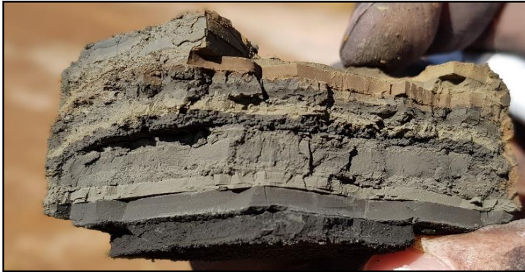
Figure 2-2: Interlayered CDR Slimes material containing fine (grey) and coarse (black) ferrochrome dust.
