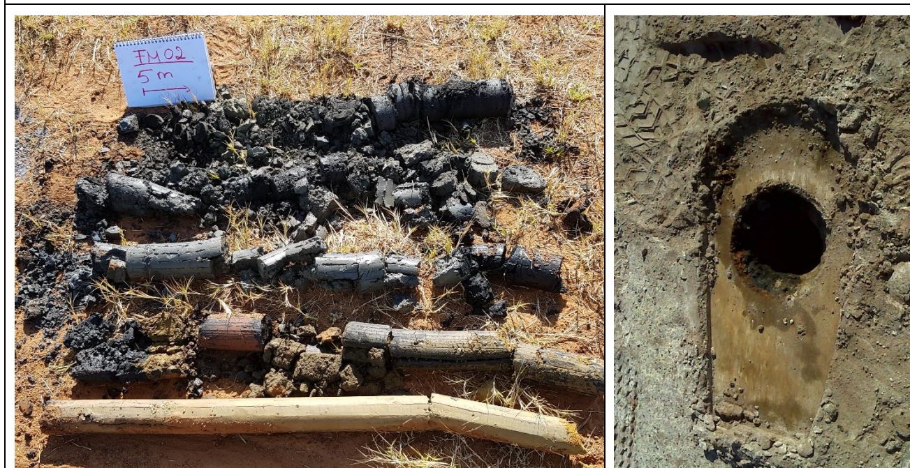
Core log of borehole MF02 with a depth of 5 m.
