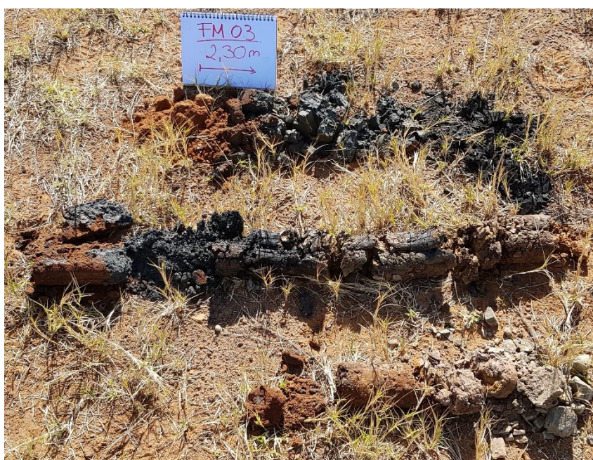
Core log of borehole MF03 with a depth of 2.3 m.
